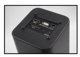
The interface of this inspection microscope is a user-friendly. From this interface, user can turn On/Off their microscope, slot in SD card, and connect mouse to control live view function.
